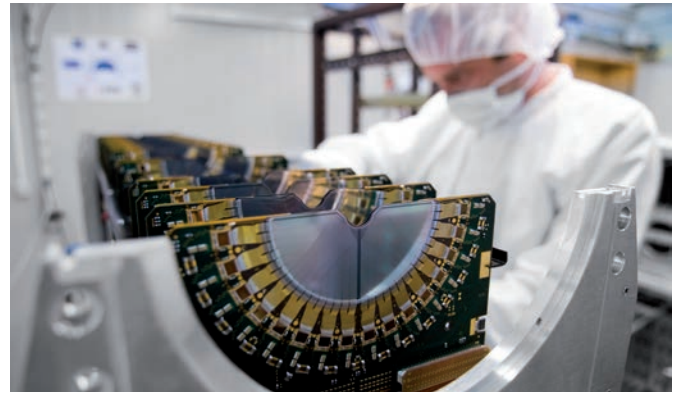
CERN - Assembling the last module of the vertex locator for LHCb. Photograph: Maximilien Brice. © 2007-2016 CERN. All Right Reserved.
