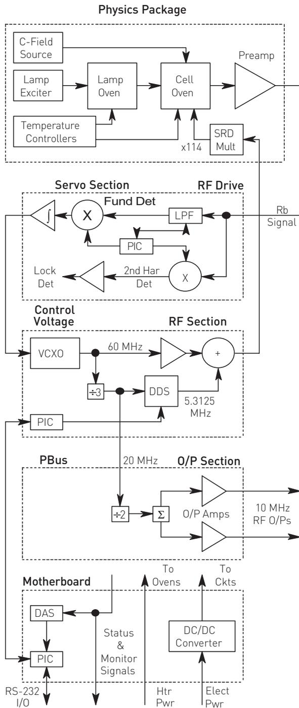
FIGURE 4 Block Diagram
