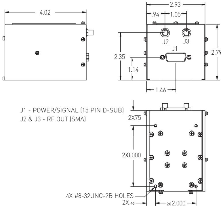
FIGURE 2 Mechanical Interface
