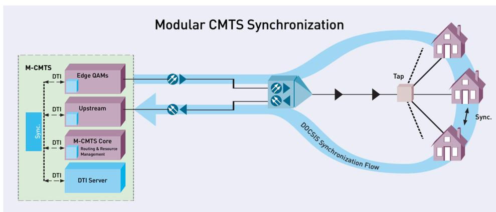
FIG. 2 M-CMTS System Flow
