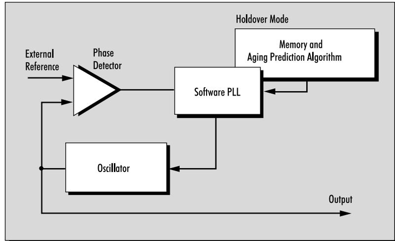
Figure 1. SmartClock Technology includes algorithms for steering the oscillator. The frequency is corrected to compensate for the effects of aging and temperature.
