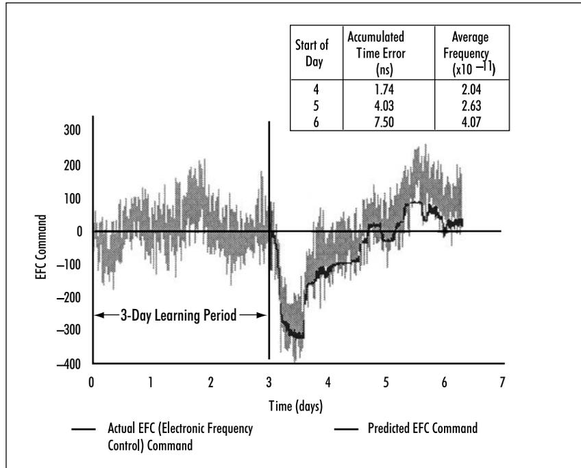
Figure 8. Example of holdover showing environmental effects.
