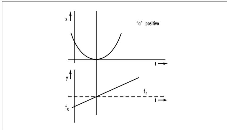
Figure A2. Positive Frequency Drift
