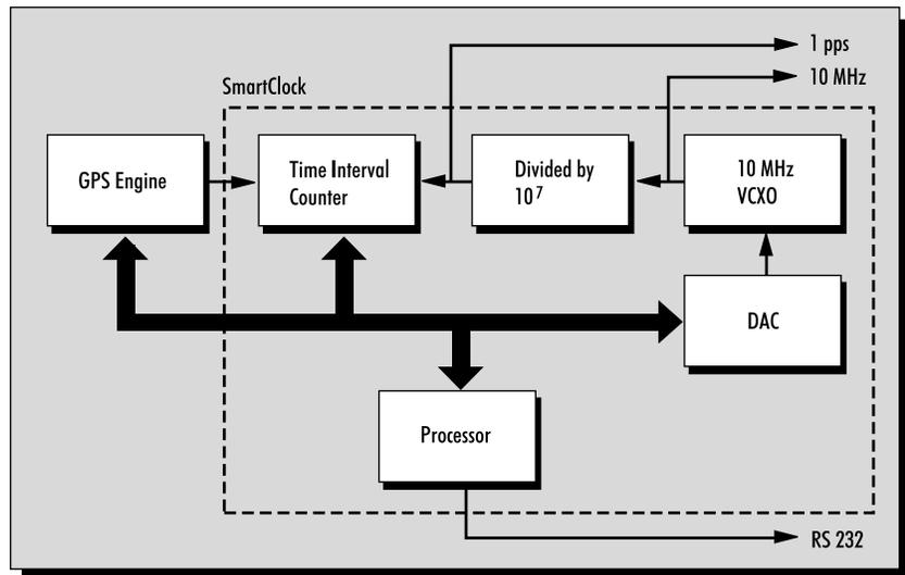
Figure 5. Block diagram for the 58503B Time and Frequency Reference Receiver.
