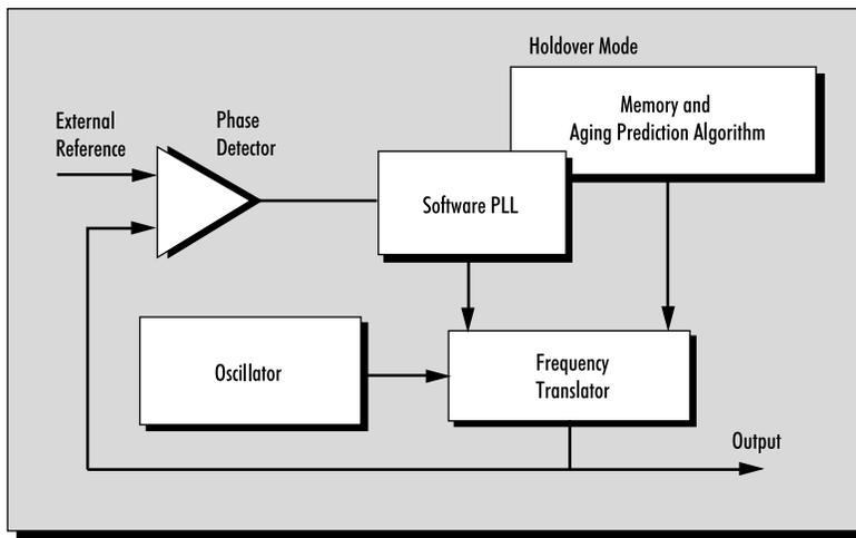
Figure 2. In this unsteered version of SmartClock, performance is improved by letting the oscillator free run and adjusting the output frequency of a high-resolution synthesizer.
