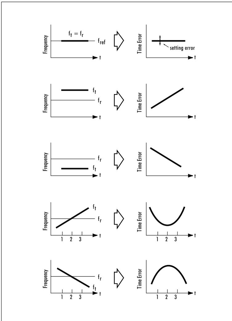
Figure A4. Frequency offsets and resulting time errors.
