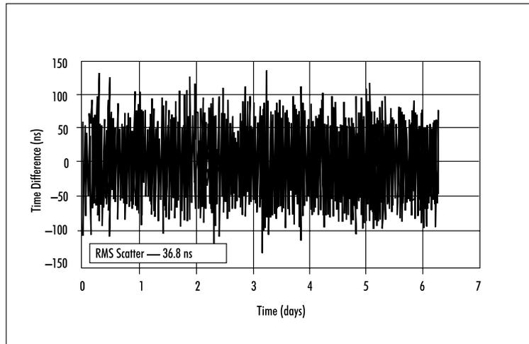
Figure 3. Raw timing data taken from a 58503B Time and Frequency Reference Receiver with the SmartClock filter disabled. The plot shows measurements of the time difference between the 1-pps output from the 6-channel GPS engine and that from an HP 5071A Primary Frequency Standard versus time. The measurements were taken over a period of six days.
