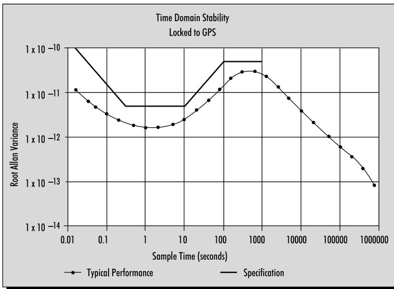
Figure 6. Root Allan Variance of the SA filtered time difference data measured by a 58503B GPS Time and Frequency Reference Receiver.
