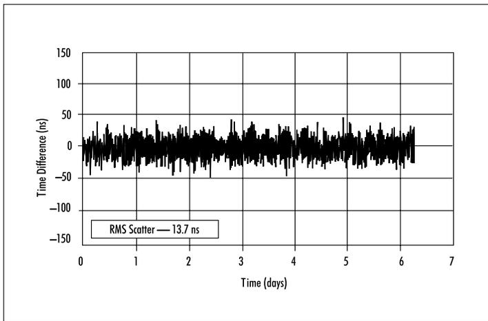
Figure 4. Time interval measurement data taken by measuring the 1-pps output of the 58530B Time and Frequency Reference Receiver against the HP 5071A Primary Frequency Standard showing the effect of the SmartClock filter reducing overall scatter to less than 16 nanoseconds rms.
