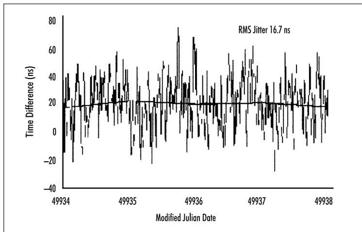
Figure 7. Direct measurement of the 1-pps output of the 59551A GPS Synchronization Module against the USNO master clock. The smooth line is a daily fit.
