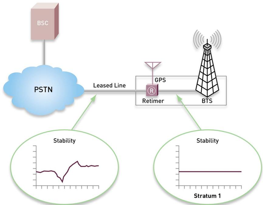
**FIG. 2** Retiming at the BTS allows the transmitter to lock its carrier frequency to a stratum one reference signal, improving call hand-offs. This prevents timing viruses and transients increasingly present on the backhaul facility from negatively impacting BTS performance.
