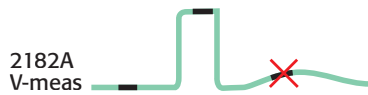
Figure 2. Heat generated by the pulse in the DUT or contacts may corrupt the third measured point, so it may be discarded.
