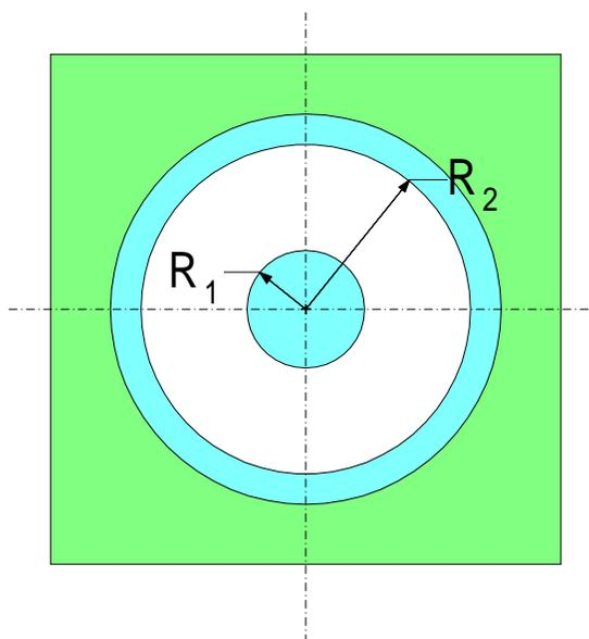
Figure 3: Surface resistance and surface resistivity measurement configuration for concentric ring electrodes.
