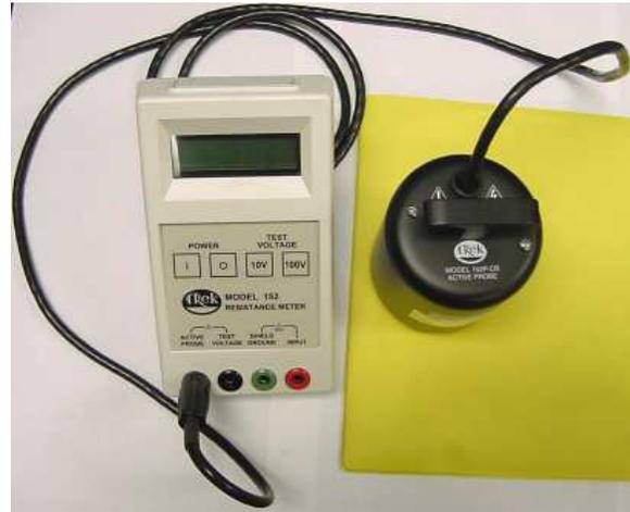
Figure 4: Surface resistivity measurement setup.
