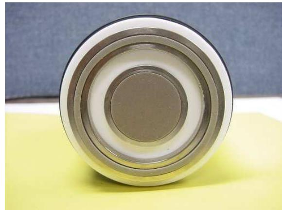
Figure 5: Concentric ring probe.
