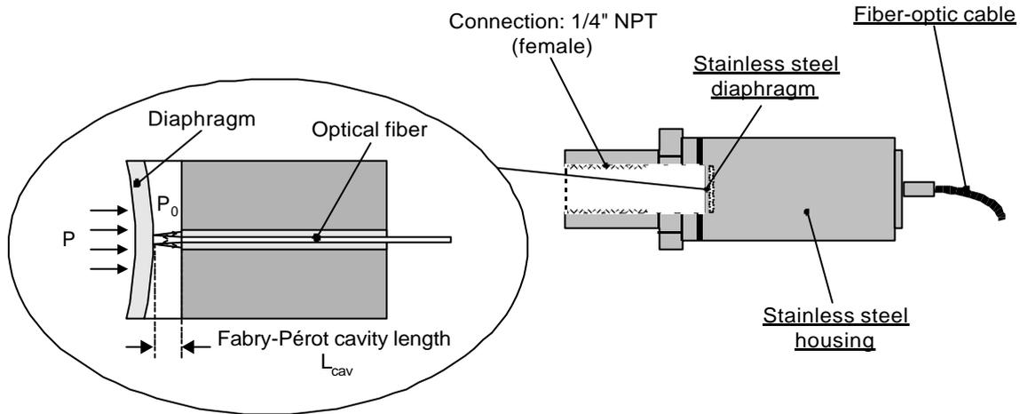
The geometry and material of the transducer are selected in order to obtain a linear relationship between the deflection of the diaphragm and the applied pressure.
