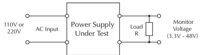
**Figure 1.** Monitoring the output of a switching power supply.
