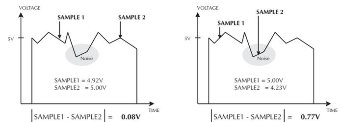
Figure 4a. Good result from multiple samples. Figure 4b. Bad result from multiple samples.
