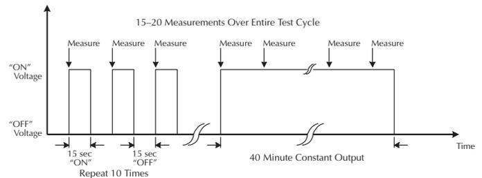
**Figure 2.** Typical burn-in test cycle.
