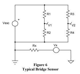
For the typical bridge sensor shown above, the differential output voltage (V1-V2) there has an inherent common mode voltage, which is typically 1/2 the excitation voltage with an additional common mode voltage component equivalent to the voltage difference between the field ground and DAS ground.
