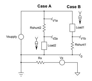
Figure 5 Current Measurements; Case A & Case B
