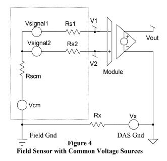
The wiring between a field sensor and its associated signal-conditioning module is subject electro-magnetic induced voltages. These induced voltages can add both an additional common mode voltage source and a differential input error voltage. Analysis of this phenomenon is beyond the scope of this document.
