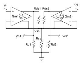
Figure 3 Simplified Model of Differential Pair
