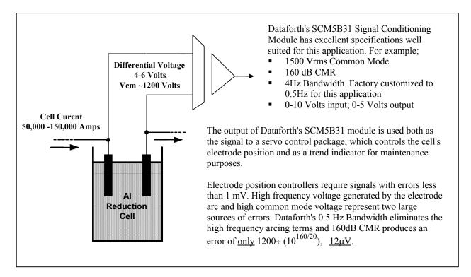
Figure 8 Measuring Al Reduction Cell Voltage
