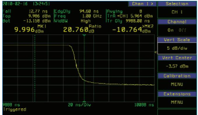
The markers show that the break point occurs approximately 20dB below the top of the pulse, equating to about 1% of the pulse power. With this in mind it should be noted that a pulse fall time is normally measured between the 90% and 10% levels, and so will not be influenced by this characteristic.
