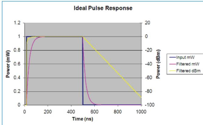
The leading edge compression and trailing edge expansion is very clear when the log scale is used. In linear mW, the leading and trailing edges appear symmetrical.
