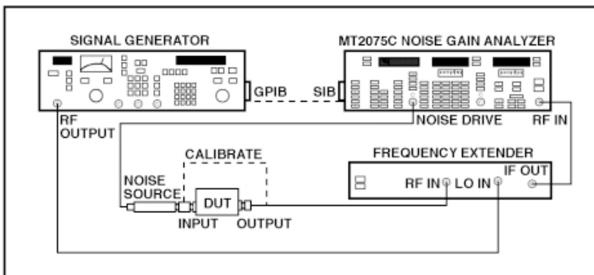
Figure 2: Noise figure measurement setup using a frequency extender.
