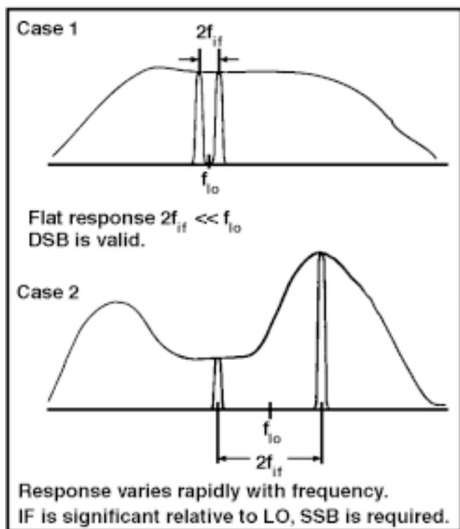
**Figure 5:** Conditions indicating validity of a DSB measurement.
