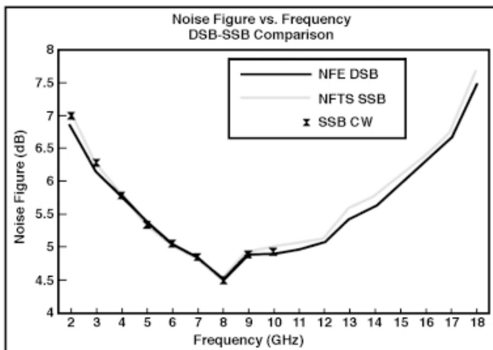
**Figure 6:** Comparison of measured single and double sideband noise figures of a 2 to 18 GHz amp using a frequency extender, a noise figure test set, and an SSB block downconverter.
