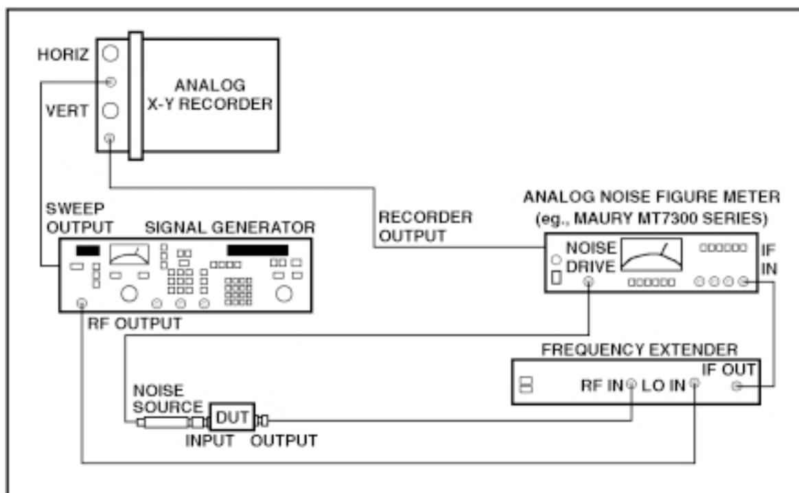
**Figure 7:** Typical noise figure measurement setup using a frequency extender and an analog noise figure meter.
