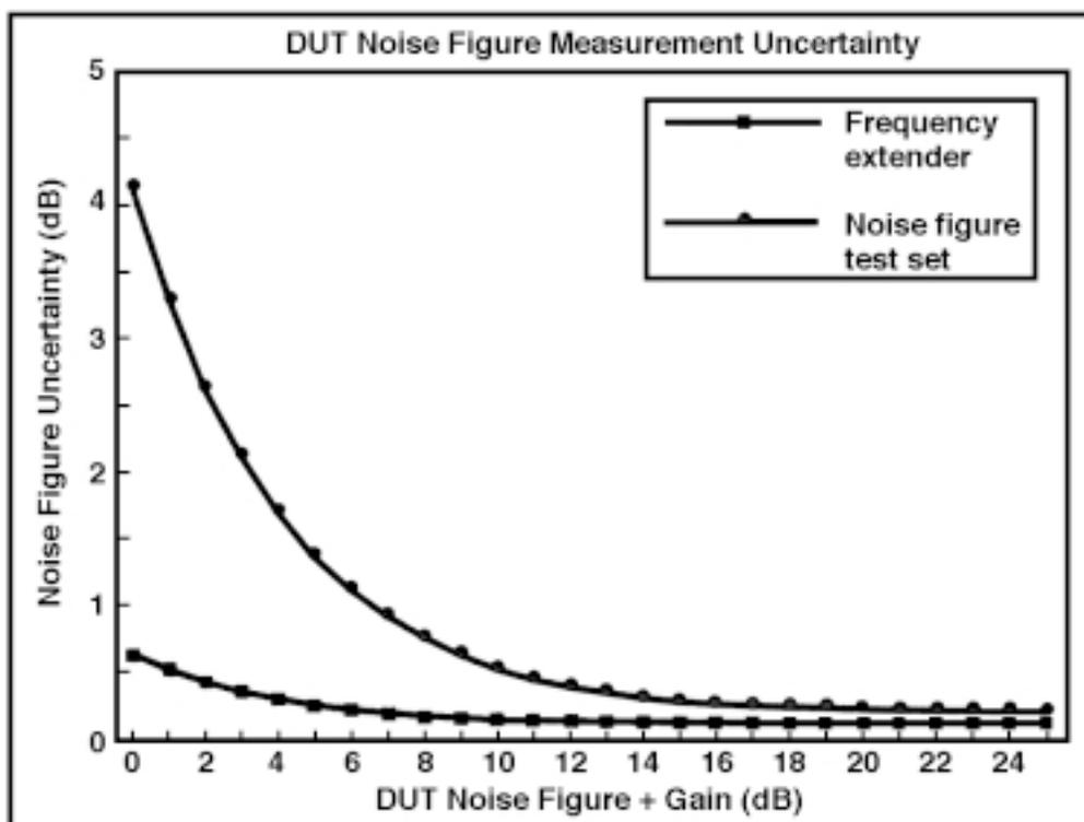
**Figure 3:** The effect of measurement system noise performance on measurement uncertainty as a function of noise figure and gain of the Device-Under-Test.
