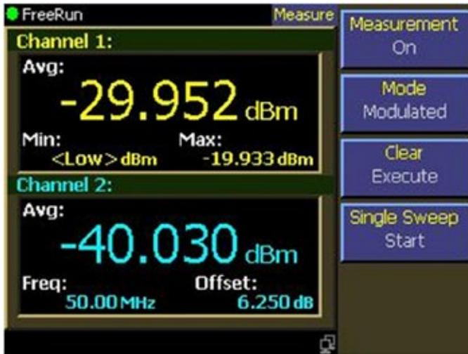
Fig. 6: Text display of a modulated mode using 2 channels on Boonton 4540
