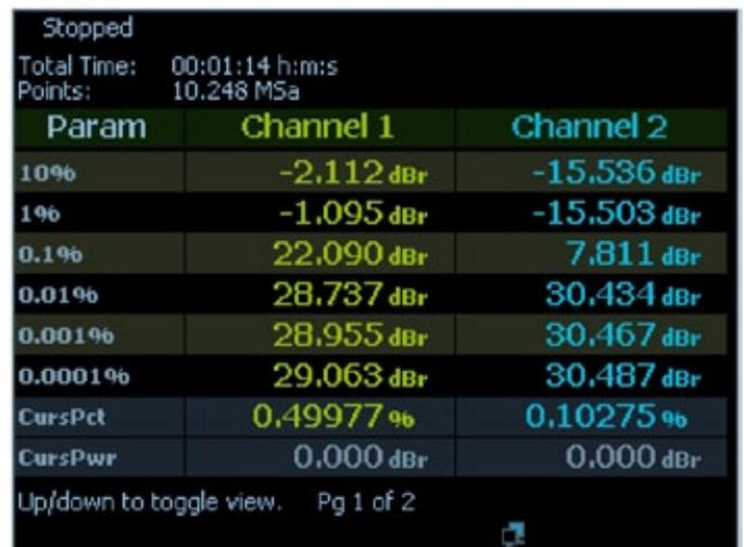
Fig. 8: Text display of a statistical measurement on Boonton 4540
