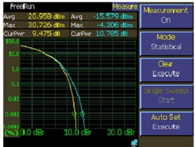
Fig. 7: Graphical display of a statistical measurement on Boonton 4540
