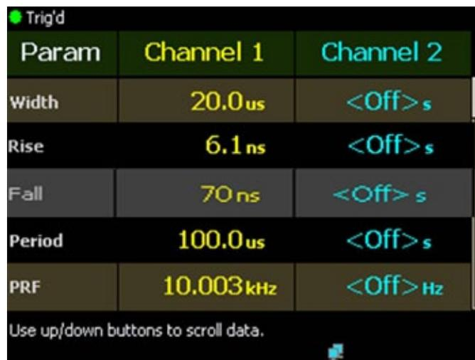
Fig. 5: Boonton 4540 numerical (Text) display of a pulse measurement
