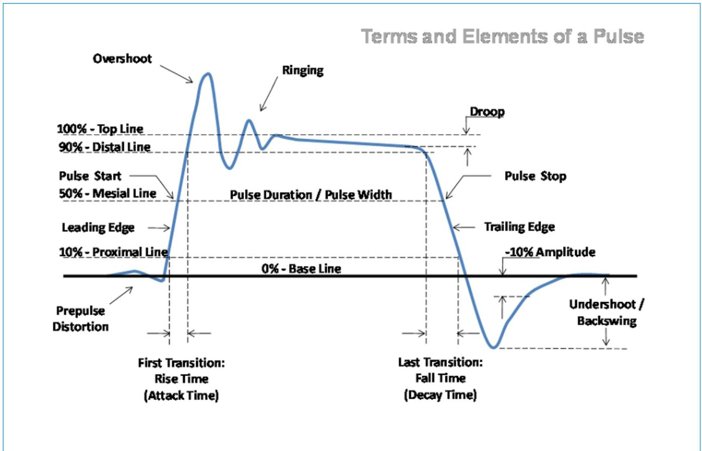
Fig.3 : Analysis of a simple pulse measurement
