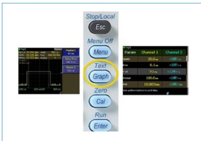
Fig. 1: "Graph/Text" button toggles to numerical display of the same measurement
