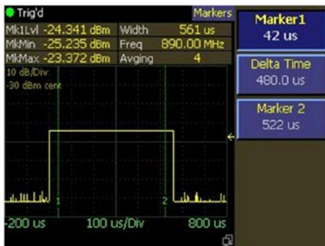
Fig. 4: Boonton 4540 graphical display of a pulse measurement
