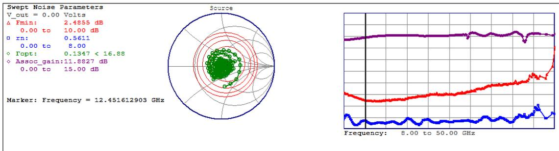
Typical 8-50 GHz single-sweep measurement using a Maury MT7553B01 Noise Receiver Module and a Maury MT984AU01 Automated Tuner with the Agilent's PNA-X.
