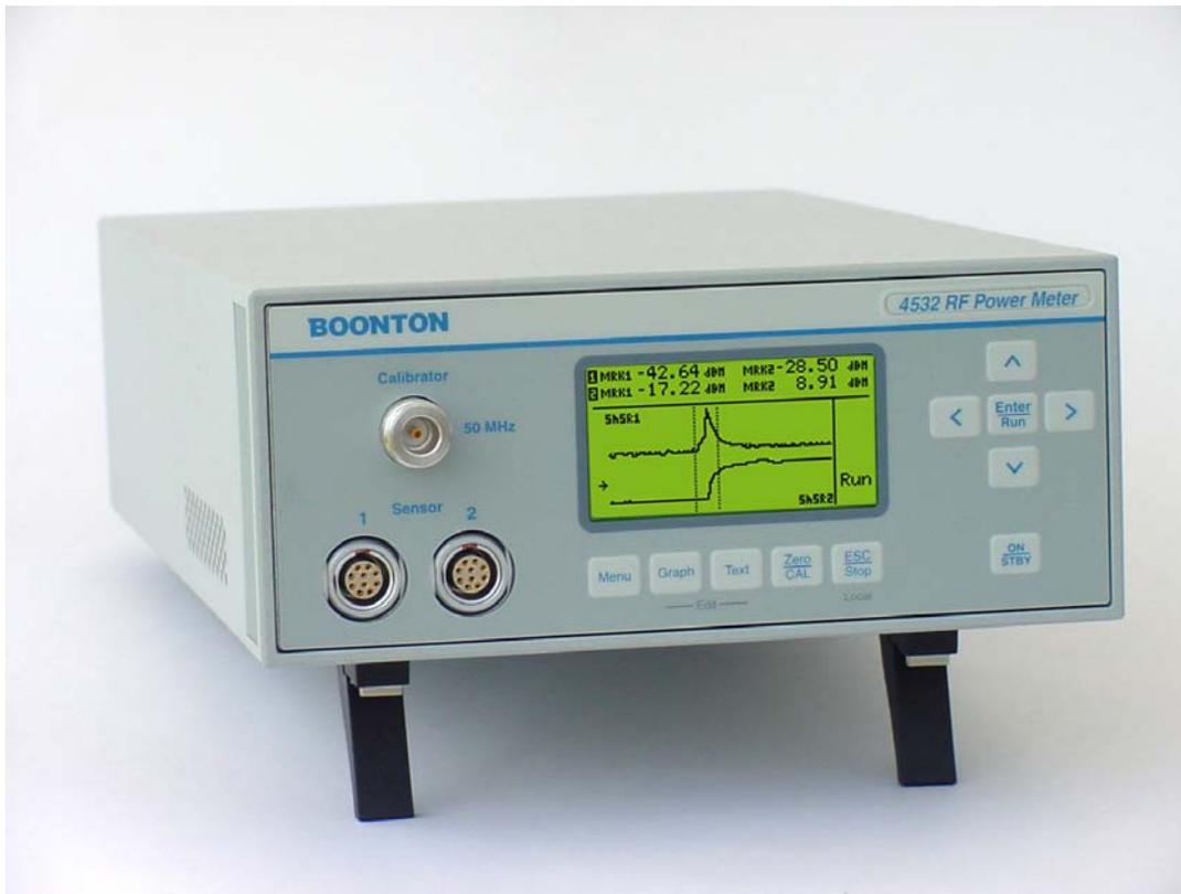
Boonton Model 4530 RF Power Meter now includes operating modes that save power readings into a memory buffer and this feature is especially useful for high-speed production test applications. These modes allow the user to store sequential power readings into an onboard memory buffer as they become available, and then read the complete buffer from the instrument into the control system after the acquisition is complete.
