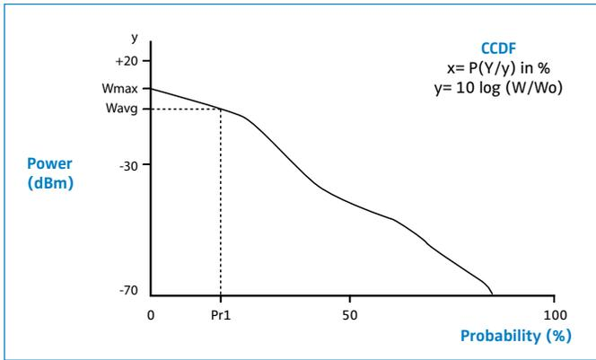
Figure 3. A CCDF with expanded time axis.
