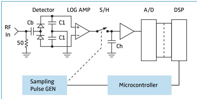
Figure 1 - Simplified view of peak power measurement system.
